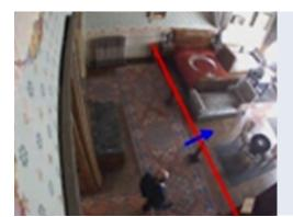
Vi-System rule "Person crossing a line", configured along a railing that marks an off-limits zone. Movement by a person across the line is detected by Vi-System and an alert is generated to notify the security team.
